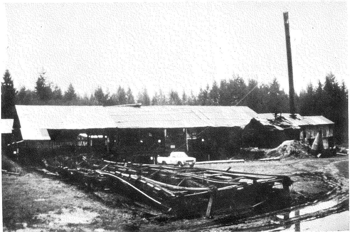
View of the sawmill, January 1992. The remains of the green chain are in the foreground.
